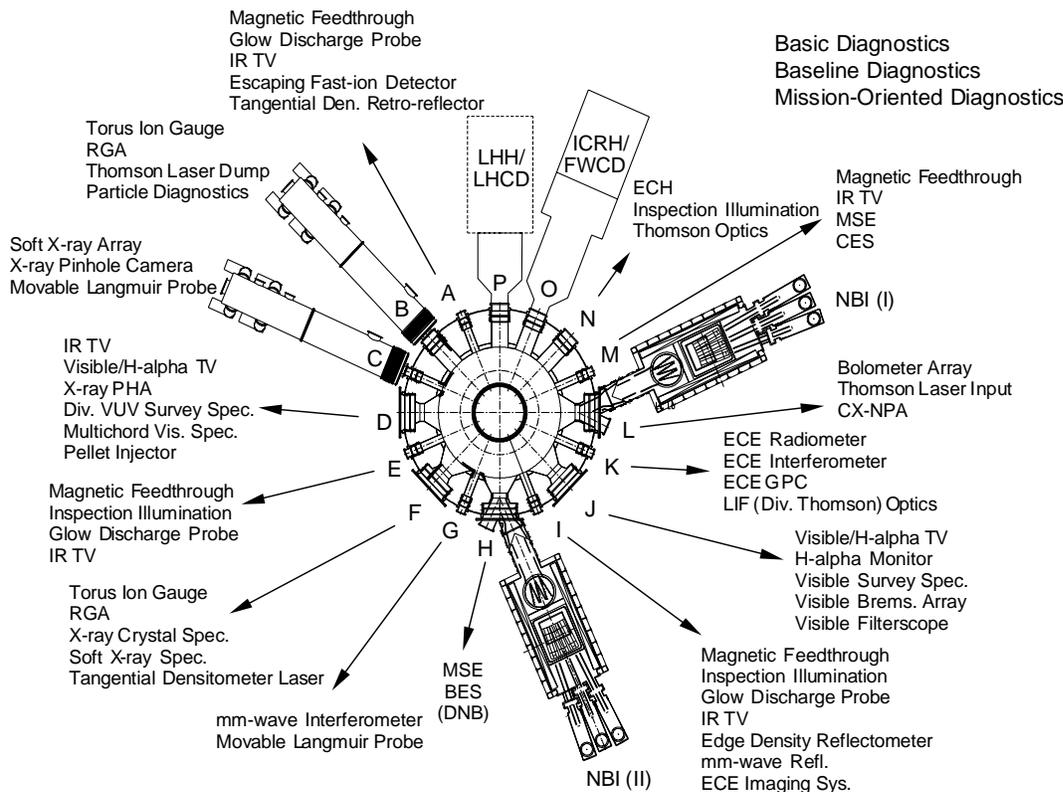
**Figure 6.** Layout of the KSTAR heating and diagnostic systems.
