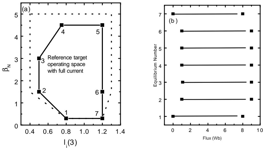
**Figure 3.** (a) Updated steady state target operating space in the  $\beta_N - I_i$  plane. Inside the solid line is the target operating space with full plasma current (2 MA) and full shape, while inside the dotted line is the extended operating space with possibly reduced plasma current. (b) Operation window at the seven corners of the target operating space.
